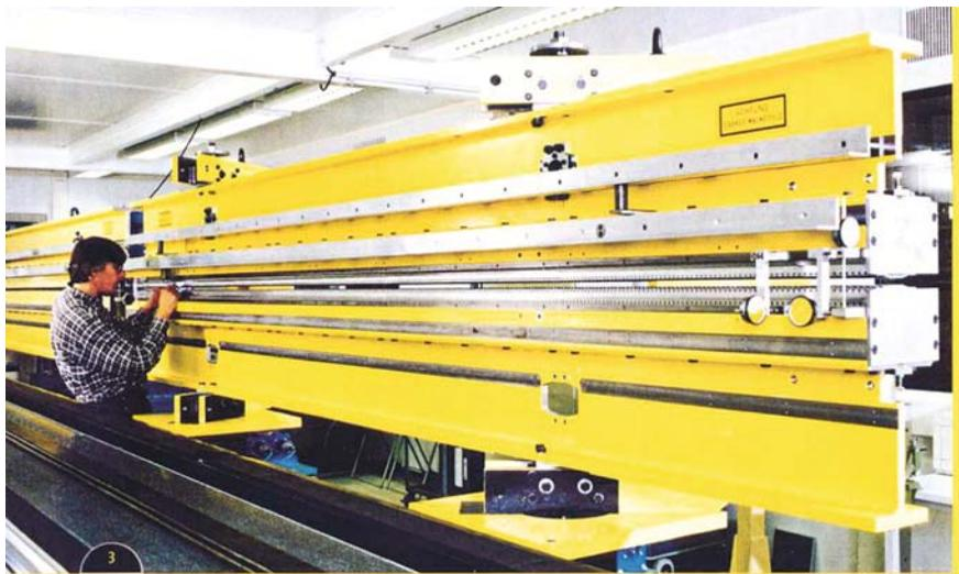
Fig. 8.12. Photo of a FLASH undulator magnet
