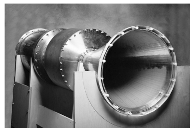
FIGURE 10.21 Bofors HPM Blackout system: pulse generator, vircator, and horn antenna. (With permission.)
