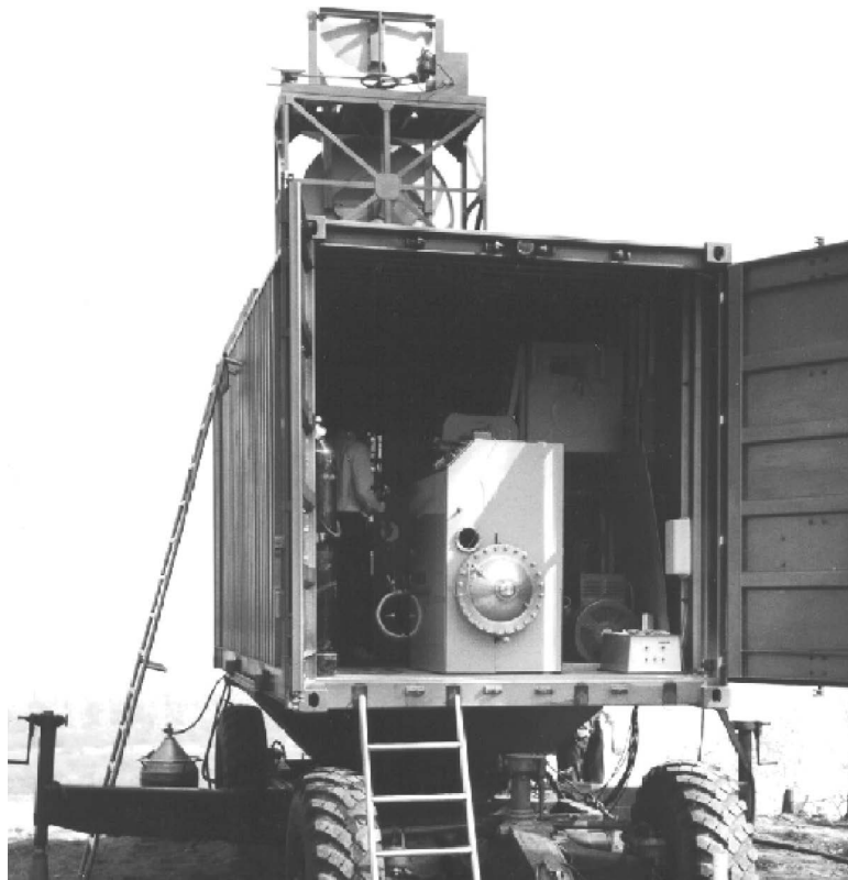
FIGURE 2.16 Transmitter cabin for the NAGIRA system. Most prominently, note the back end of the SINUS pulsed power generator. The motor generator supplying prime power is seen to the lower right. The lower dish on the roof is the transmitting antenna, while the upper dish is the receiving antenna.
