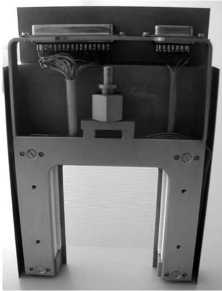
Fig. 6.3. Harp detector [33], shown from the back, provided for emittance measurements. The detector consists of 60 W-Re wires with a diameter of 0.1 mm having a spacing of 1 mm
