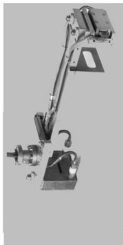
Fig. 6.2. Mechanical components of an emittance measuring system. See Appendix 6.A for the dimensioning of motor driven feedthroughs
