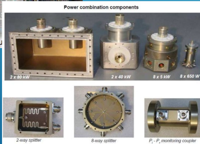
SOLEIL SSA: Frequency: 352 MHz Output power: 180 kW 726 × 315 modules in 4 towers. 2 × Si LDMOS transistors per module
