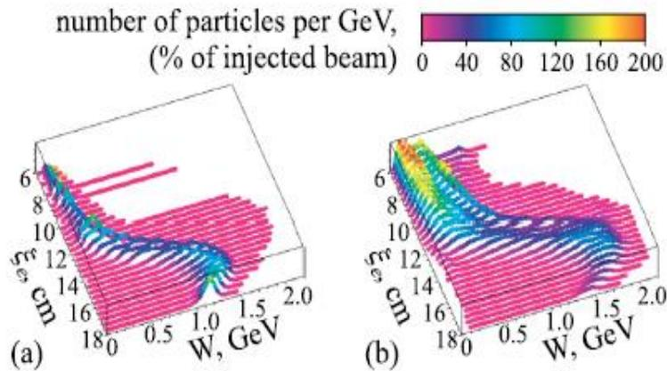
Final energy spectra for (a) electrons and (b) positrons as a function of injection delay  $n_e$  with no beam loading effect taken into account
