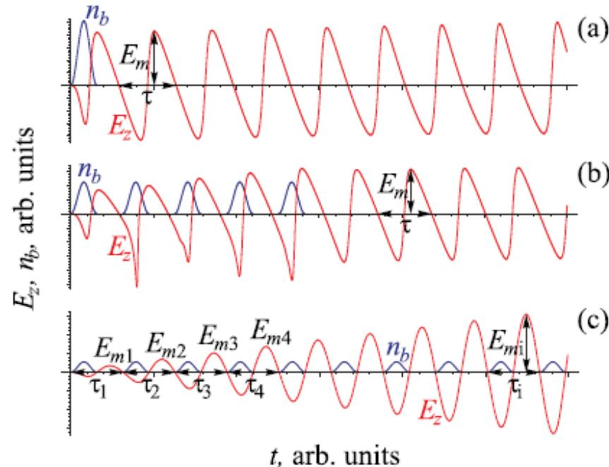
Location of the measured wave periods for the single bunch of variable charge (a), the train of 5 bunches (b), and the infinite bunch train (c).
