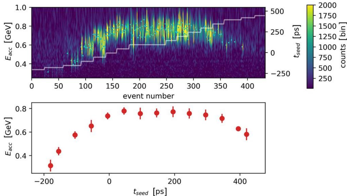
Top: waterfall plot of the measured electron energy spectra (right axis) during the seed scan. The value of  $t_{seed}$  is shown by the white line and the vertical axis on the right. Bottom: energy of the charge peak of the accelerated electrons as a function of seed timing.
