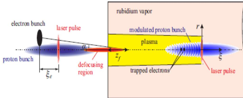
The optimum values found in simulations are: electron delay  $\epsilon_e = 11.5$  cm, injection angle  $\alpha = 2.8$  mrad, and focusing point  $z_f = 140$  cm.
