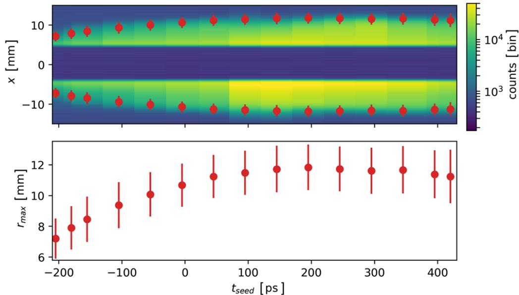
summed waterfall plot of the horizontal line-outs of the measured self-modulated proton bunch transverse distribution as a function of  $t_{seed}$ .
