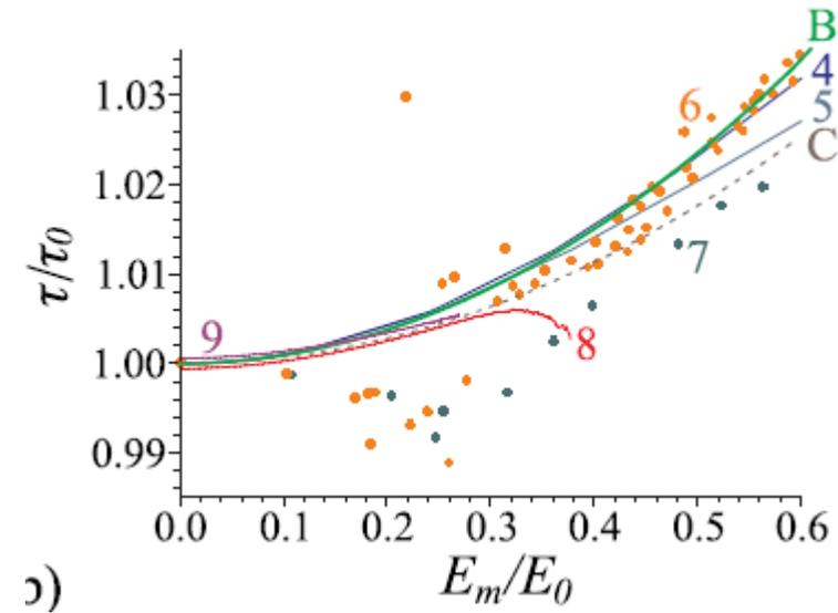
Dependence of the wake-field period on the wave amplitude for various drivers.
