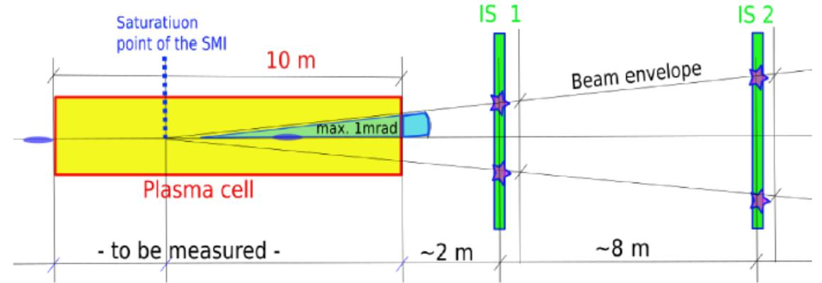
Schematic drawing of the principle behind the two screen measurement setup.
