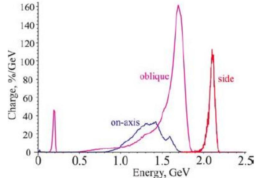
✓ The final simulated energy spectra of electrons in cases of the side, on-axis and oblique injection methods.
