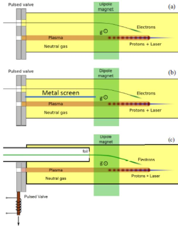
Various designs of electron beam side injection
