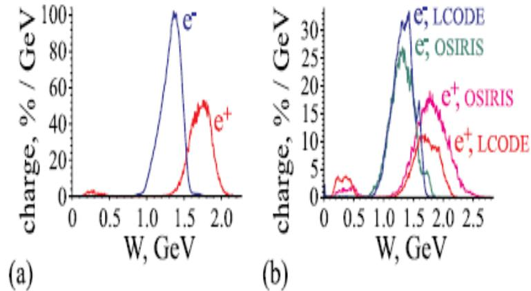
Final energy spectra of electron and positron bunches injected at the nominal delay  $\epsilon z = 16.4$  cm without (a) and with (b) beam loading.
