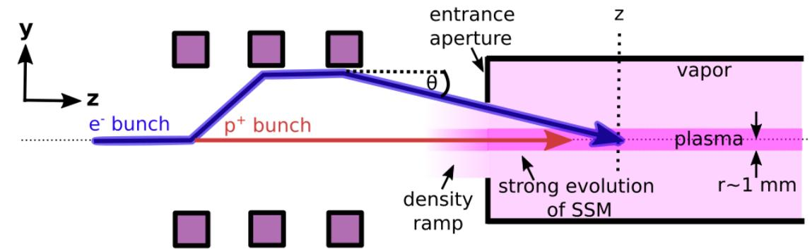
Schematic drawing of the electron injection scheme in the vertical plane (only corrector magnets are shown, see Fig. I).
