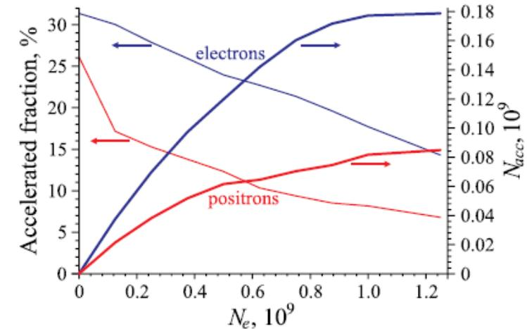
Fraction of accelerated and total number of accelerated particles  $N_{acc}$  (thick lines, right scale) versus the number of injected particles  $N_e$  for electron and positron beams.
